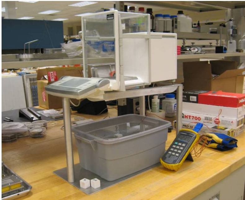
Photo No. 7 ASTM D 792 Density Specimen Being Weighed in Water (File Photo)
