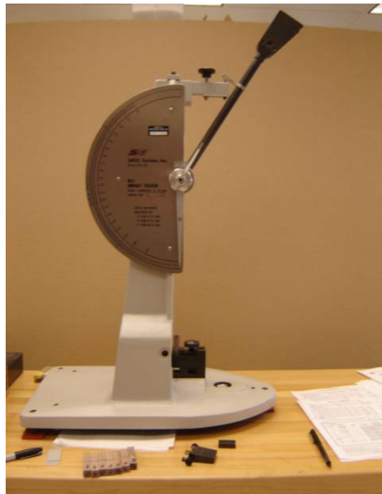
Photo No. 10 ASTM D 256 Izod Impact Test Setup (File Photo)
