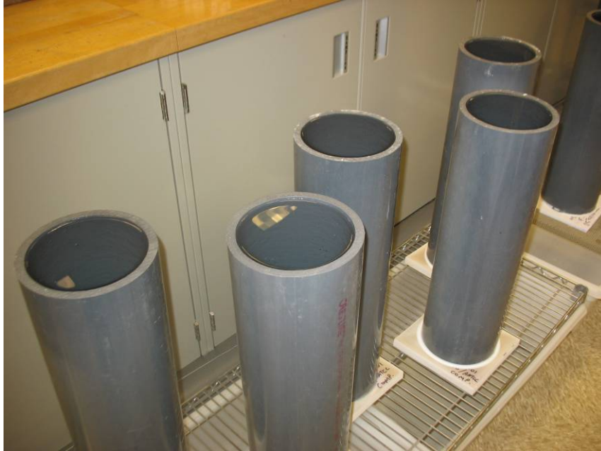
Photo No. 2 ASTM D 570-Exposed Specimens Undergoing AATCC Test Method No. 127 Hydrostatic Head Testing (File Photo)
