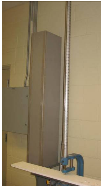
Photo No. 8 ASTM D 5420 Gardner Impact Testing Setup (File Photo)
