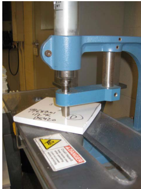
Photo No. 9 Close-up of ASTM D 5420 Gardner Impact Testing Setup (File Photo)
