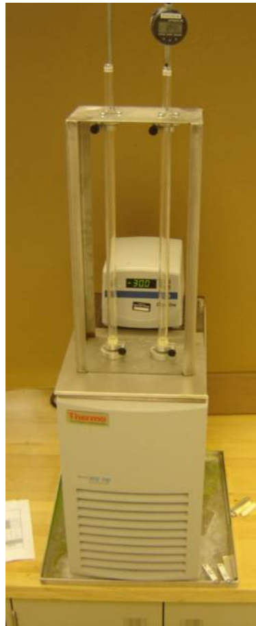
Photo No. 1 ASTM D 696 CLTE Test Setup (File Photo)
