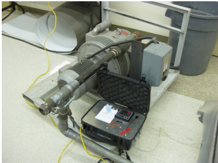
Photo No. 6 ASTM E 330 Blower and Pressure Measuring Device (File Photo)
