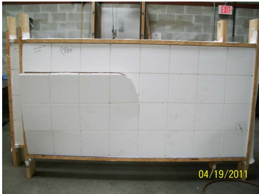
Photo No. 4 Typical ASTM E 330 Transverse Wind Load Test Specimen
